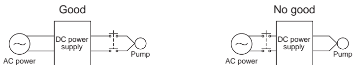
Wiring example
