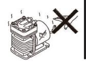
Always use a suction valve to adjust an air flow.
