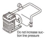
• Do not tube two or more pumps in series. It may prevent the motor from starting and lead to a burn out.
