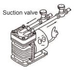
• The APN-S110 is designed for vacuum application only. Do not pressurize the discharge line of the pump.
